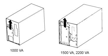
**3.** 1000 VA units. Disconnect the red battery cable on the front of the battery. Pull the battery out onto a flat, stable surface. Disconnect the black battery cable on the rear of the battery, then on the front of the battery. Disconnect the red battery cable on the rear of the battery. See "Recycling the Used Battery" on page 20 for proper disposal.
